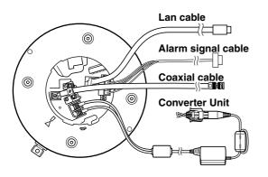
The connection cables include Alarm Signal cable, LAN cable, coaxial cable and Converter Unit.
